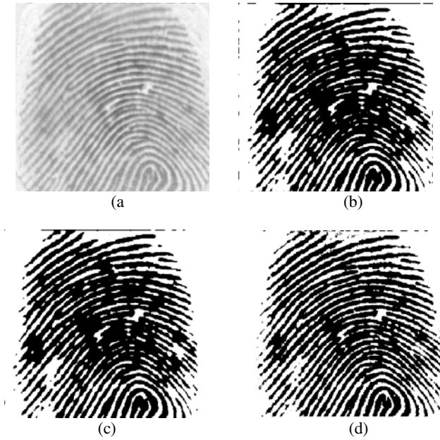
Fig. 2. Fingerprint image segmentation. (a) original fingerprint image. (b) fingerprint segmentation result using Otsu's method. (c) fingerprint segmentation result using Kapur's method. (d) fingerprint segmentation result using proposed method.
